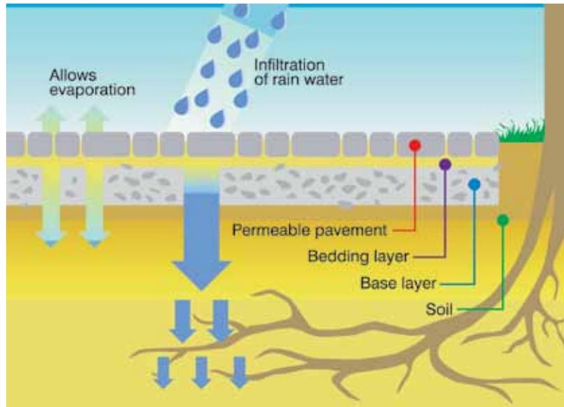
Illustration of the Unilock Permeable Pavement System
